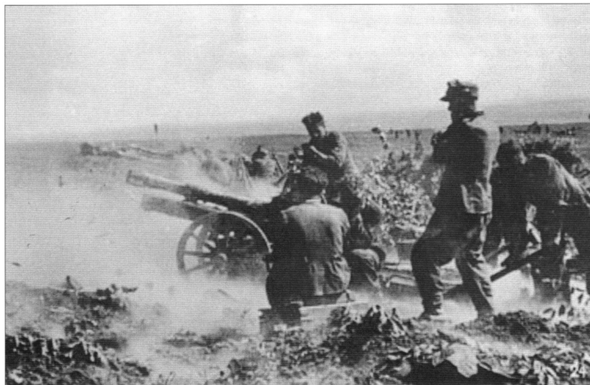
A 7.5cm Gebirgskanone in action. Note the compact size of this weapon, designed to be easily disassembled for transport by pack animals.
